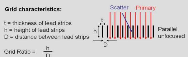
It is the ratio of the height of lead strips to the distance between the strips.
